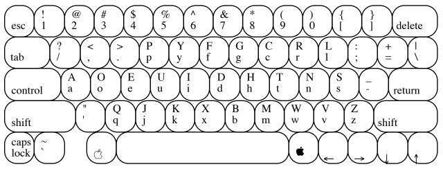
Figure 1–Dvorak DSK Layout on Early IIc Computers
