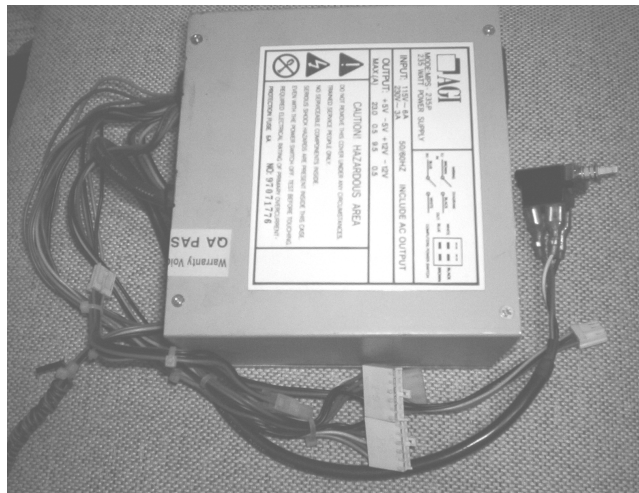
Typical AT-style power supply found in 386-Pentium computers
