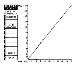
Partial frequencies need not be harmonically related. The 2-D graphic display clearly shows deviations from perfect harmonic frequencies. 'Selected' partials are indicated by solid dots.
