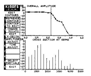
A cross section plot shows the sound's spectrum at any point in time. Note that time has scrolled forward to show the tail end of the sound's envelope. Breakpoints of all of the partials combined are shown on the overall amplitude plot.
