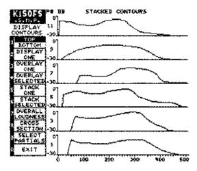
One method of working with dynamic spectral changes is to display the contours of selected partials as a 'stack' of plots. Detailed editing is performed on one such plot expanded to cover half the screen.
