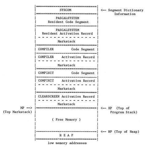
FIGURE 5 DETAIL OF USER MEMORY DURING EXECUTION OF PROCEDURE "CLEARSCREEN"
