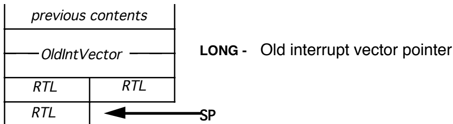
Figure 2—The Stack on Entry to ShutDown
