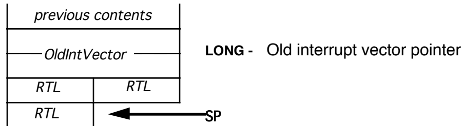
Figure 3—The Stack on Entry to Reset
