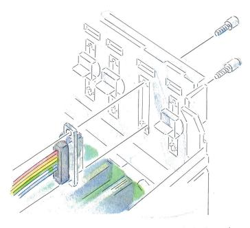
Figure A-13 Anchoring the cable connector to the back panel
