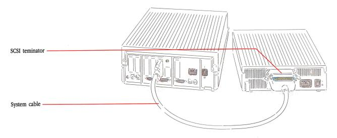
Figure A-21 The completed connection
