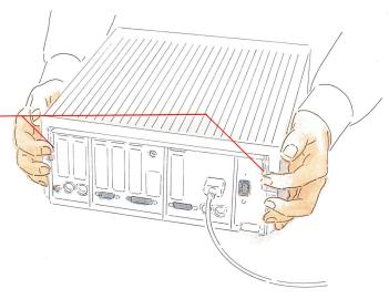
Figure A-10 Removing the computer's lid
