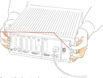
Figure A-5 Removing the computer's lid
