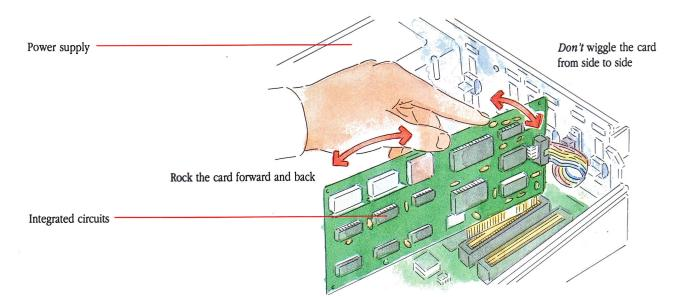
Figure A-15 Inserting the card
