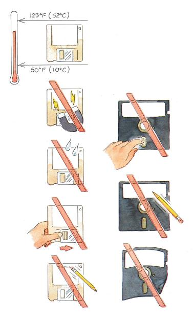
Figure 4-15 The proper care and handling of disks
