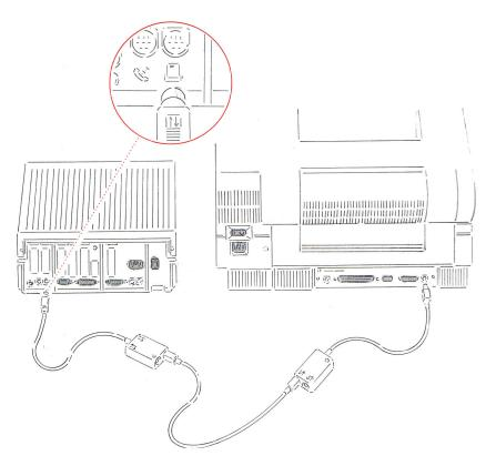
Figure A-2 Connecting a LaserWriter printer
