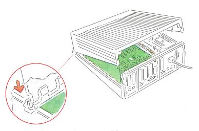
Figure A-17 Replacing the computer's lid
