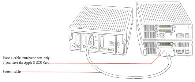
Figure A-22 Connecting the cable terminator and the system cable
