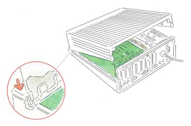
Figure A-9 Replacing the computer's lid
