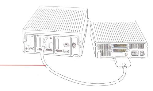
Figure A-20 Connecting the system cable
