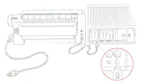
Figure A-1 Connecting an ImageWriter printer
