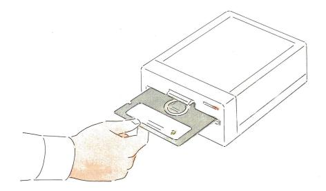
Figure 4-4 Inserting a 5.25-inch disk
