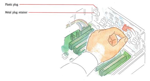
Removing the plastic plug Figure A-12
