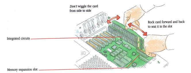
Figure A-8 Inserting the card
