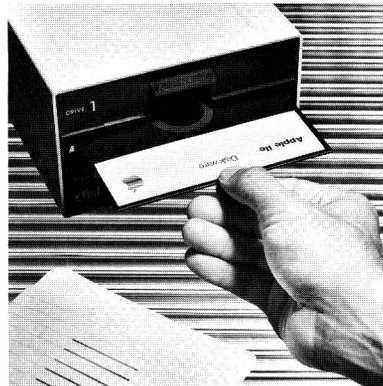
Figure A-1. How to Insert the MASTER Disk into the Disk Drive
