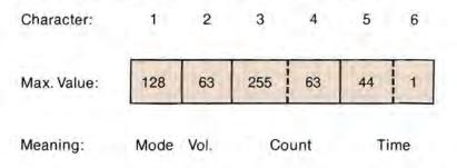
The count and time values are two-byte integers, with the low-order byte first. The maximum values shown for these parameters are the two-byte values: the low-order byte of the time value can range from  $\emptyset$  to 255, but the maximum time value is 30 $\emptyset$ . This is obtained by adding a low-order byte of 44 to the value of a high-order byte of 1, that is, \$100 or 256.
