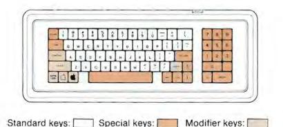
The special keys are the ESCAPE, TAB, RETURN, the spacebar, and the four arrow keys on the main keyboard, and all keys on the numeric keypad. The special keys always generate the same ASCII codes, regardless of the condition of the SHIFT and CONTROL keys. The keyboard layout table does not define codes for these keys.
