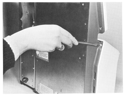
Figure 2-4. Removing the cover screws
