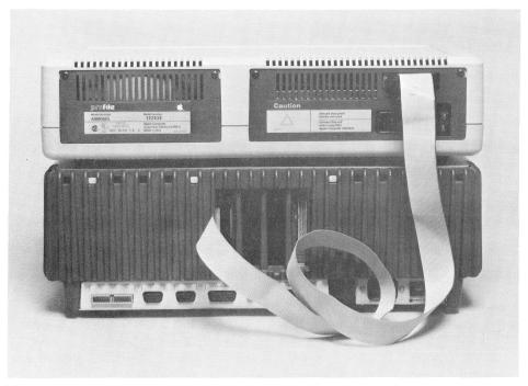
Figure 2-9. Connecting the Profile hard disk drive
