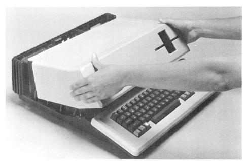
Figure 2-5. Removing the cover
