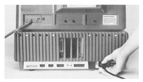
Figure 2-1. AC connector at the rear of the Apple III
