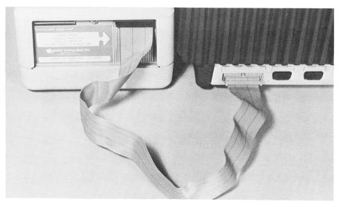
Figure 2-3. Connecting the Apple Disk III
