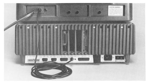
Figure 2-2. Connecting the video monitor
