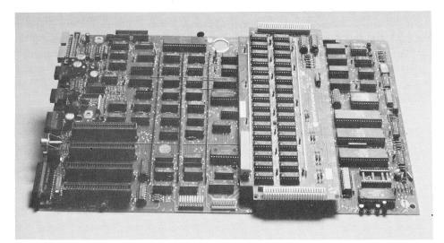
Figure 1-9. Apple III circuit board
