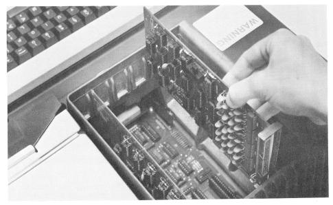
Figure 2-8. Plugging in a board
