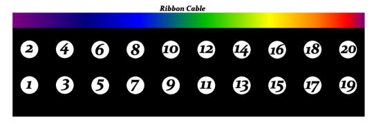
The above diagram is looking at the back of the plug (top side, where ribbon cable connects.
