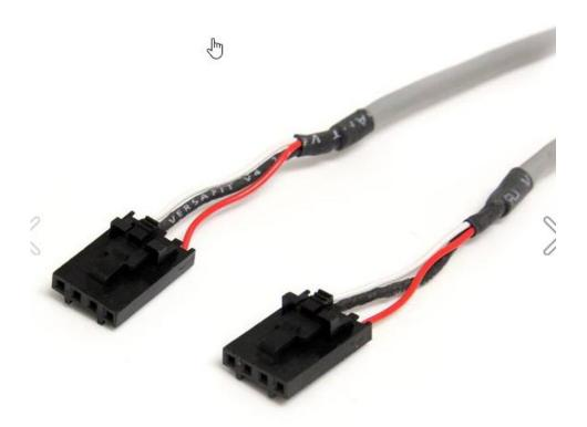
I scavenged the ends from an MPC2 styled CD-ROM audio cable. Just push on the metal locking tab on the back of connector and pull out the wires
