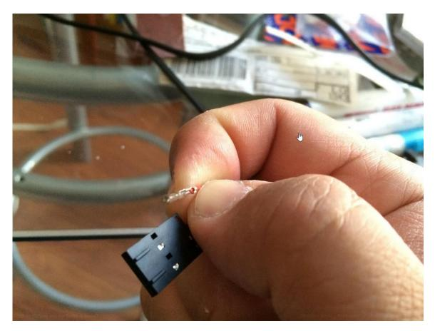
This is the end of the wire that will slide over the original battery lead on the logic board
