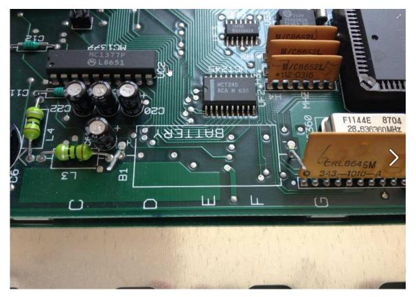
Snip off the original battery closest to the ends of the battery to leave as much as the existing leads as possible on. Then straighten the leads.
