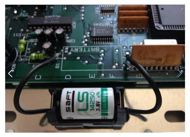
Use heat shrink tubing to insulate. Best to use a red and black tubing to color code. I didn't have red on hand so I just used black. Then bend the leads on the bottom out the sides so it's parallel to the battery holder. Slide the ends of the wires onto the leads on the logic board
