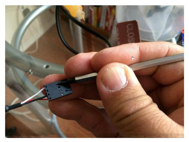
Push on locking tab with a small screw driver and pull the wire out.
