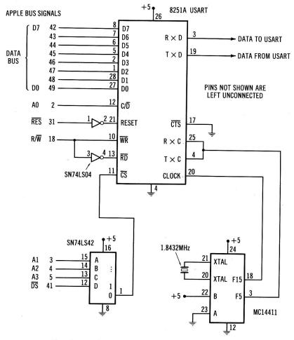
Fig. 7-10. Simple USART-to-Apple interface circuit schematic.
