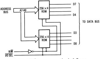
Fig. 7-11. A 256-byte memory expansion circuit diagram.
