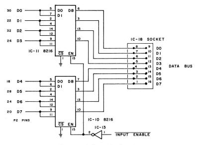
Fig. 5-5. Bus buffer circuit schematic.
