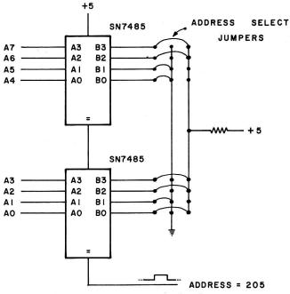
Fig. 2-18. Two SN7485 comparators used to detect address 205.
