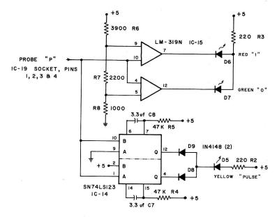
Fig. 5-3. Logic probe circuit schematic.
