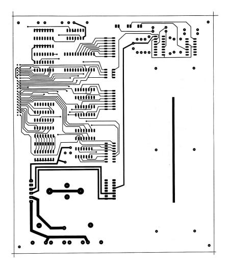
Fig. E-2. Printed-circuit board artwork for solder side of interface breadboard (reverse reading).
