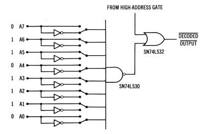
Fig. 2-5. Programmable gate used for device address decoding. (High address section is equivalent.)
