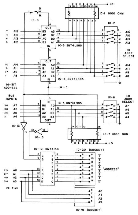
Fig. 5-4. Address decoder circuit schematic.
