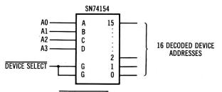
Fig. 7-4. Using DEVICE SELECT to enable a 16-address decoder.
