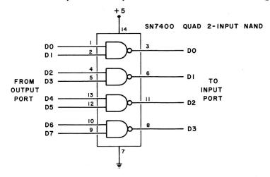
Fig. 6-16. Schematic for the SN7400 NAND gate test circuit.
