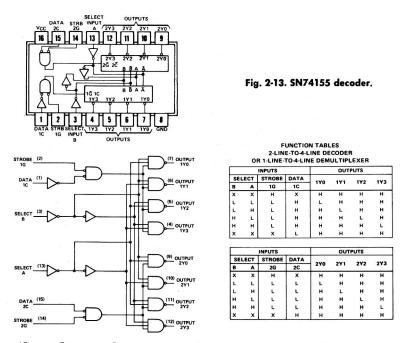
ers, depending on the type you choose, may have additional inputs, enable lines, and outputs. Examples are shown in Fig. 2-11 for the SN74LS138 decoder and in Fig. 2-12 for the SN74154 decoder. The SN75155 decoder has also been included (Fig. 2-13) since it has two
