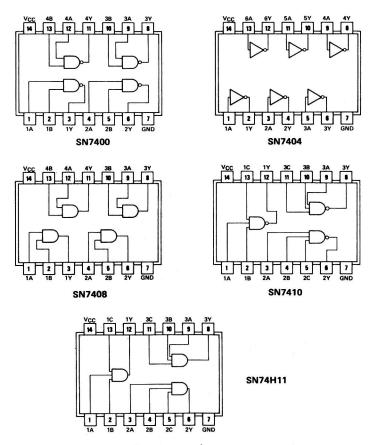
Fig. 2-1. Inverter and various AND/NAND gate pin configurations.
