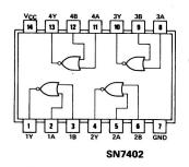
Fig. 6-3. SN7402 NOR-gate pin configuration.
