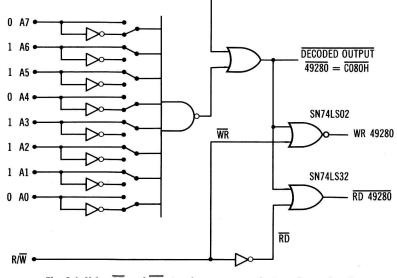
Fig. 2-6. Using RD and WR signals to generate device select pulses for device synchronization.
