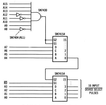
Fig. 2-16. An improved device selection circuit.
