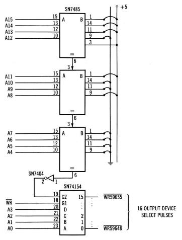
Fig. 2-19. Comparators and decoders used for address selection.
