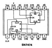
Fig. 6-5. SN7402 and SN7474 chip pin configurations.
