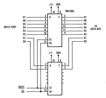
Fig. 3-10. Typical input port constructed using SN74365 chips.
