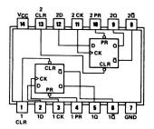
Fig. 6-20. SN7474 dual D-type flip-flop chip pin configuration.
