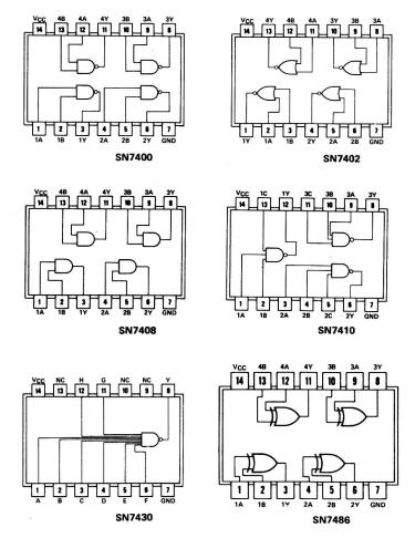
Fig. 6-17. Pin configurations of some standard gates.
