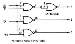
Fig. 6-4. Function pulse-generation circuit.
