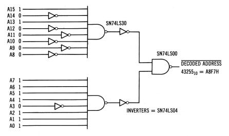
Fig. 2-2. Gating circuit used to decode address 43255 or A8F7H.
