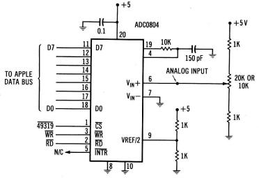
Fig. 6-24. ADC0804 interface circuit schematic.
