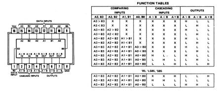
Fig. 2-17. SN7485 four-bit magnitude comparator chip.
