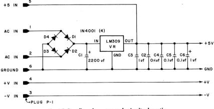
Fig. 5-2. Breadboard power-supply circuit schematic.
