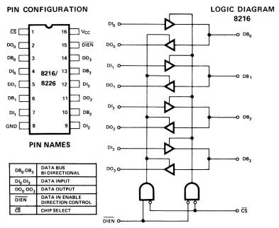
Fig. 5-6. The 8216 bus buffer chip pin configuration.
