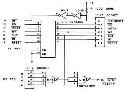
Fig. 5-7. Control circuit schematic.
