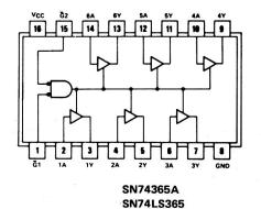
Fig. 6-7. SN74365, or DM8095 threestate buffer chip pin configuration.
