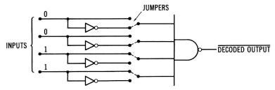
Fig. 2-4. A simple 4-input gate that can be programmed for 1's and 0's.
