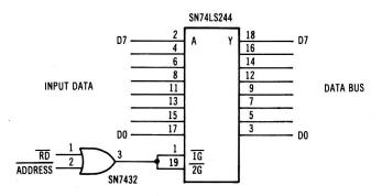
Fig. 3-12. Input port configured with an SN74LS244 chip.
