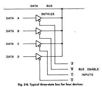
the SN74126, is a pin-for-pin replacement for the SN74125, except that it is enabled with a logic one and disabled with a logic zero. These chips serve to illustrate the action of three-state devices, but they are not generally found in computer interface circuits, since more useful devices are available.
