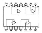
Fig. 3-7. SN74125 bus buffer chip pin configuration.
