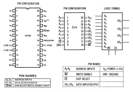
Fig. 1-2. Pin configuration for 2708 1K  $\times$  8 PROM and 2114 1K  $\times$  4 R/W memory.
