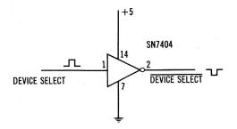
Fig. 6-13. Simple device-select pulse-inverter circuit.
