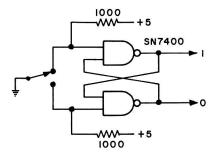
Fig. A-3, two outputs are available. With the switch in the position shown, the normal logic states are shown at the outputs of the two gates. When the switch is moved to the other position, the outputs of the NAND gates will switch. It is suggested that a momentary switch be used in the pulser circuits.
