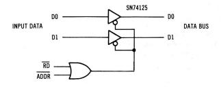
Fig. 3-13. Two-bit input port.
