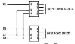
Fig. 2-10. Decoder enable inputs used with WR and RD to generate device select signals.
