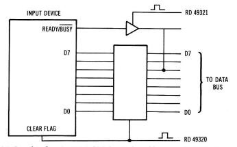
Fig. 4-5. Complete flag circuit in which flag is cleared by computer-generated pulse.
