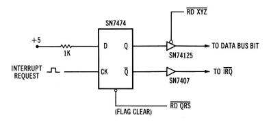
Fig. 7-5. Interrupt flag circuit diagram.
