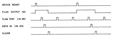
Fig. 4-8. Flag flip-flop timing diagram.
