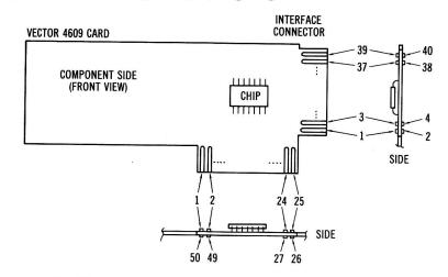
Fig. 5-13. Vector 4609 card contacts and interface contact arrangements.
