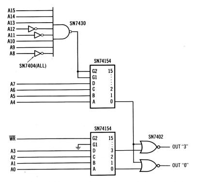
Fig. 2-15. Using SN74154 decoders and gating for absolute device address selection.
