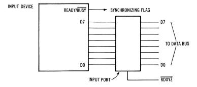
Fig. 4-1. Simple input device with synchronizing flag output.
