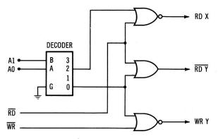
Fig. 2-8. 2-Line-to-4-line decoder used for device addressing.
