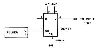
Fig. 6-21. Simple Rip-flop-based flag circuit.
