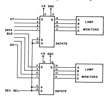
Fig. 6-10. Simple 8-bit output port schematic.
