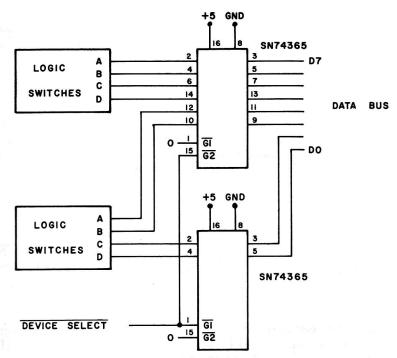
Fig. 6-8. Simple 8-bit input port.
