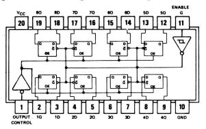
Fig. 6-14. SN74LS373 octal latch chip pin configuration.
