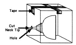
7. Standing to one side, use a pair of diagonal cutters to snip off the very tip of the CRT neck protruding through the hole.
