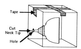
5. Standing to one side, use a pair of diagonal cutters to snip off the very tip of the CRT neck protruding through the hole.
