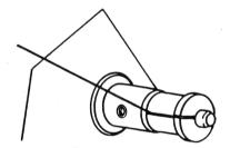
6. Keeping the wire taut, manually wind the wire onto the pulley by rotating the pulley clockwise nine revolutions.
