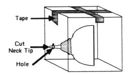
Standing to one side, use a pair of diagonal cutters to 7. snip off the very tip of the CRT neck protruding through the hole.
