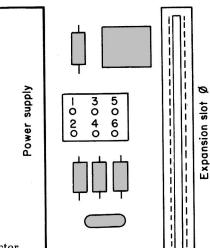
**FIG. 5–4** Pin locations on power supply connector.
