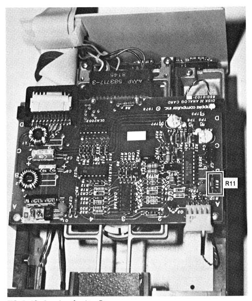
FIG. 4–19 Location of resistor R11.
