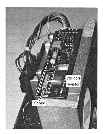
**FIG. 4–26** Variable resistor.
