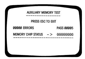
FIG. 11-11 Auxiliary memory test screen.
