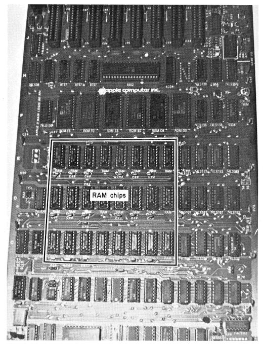
**FIG. 5–11** Location of RAM chips on the II and II+.
