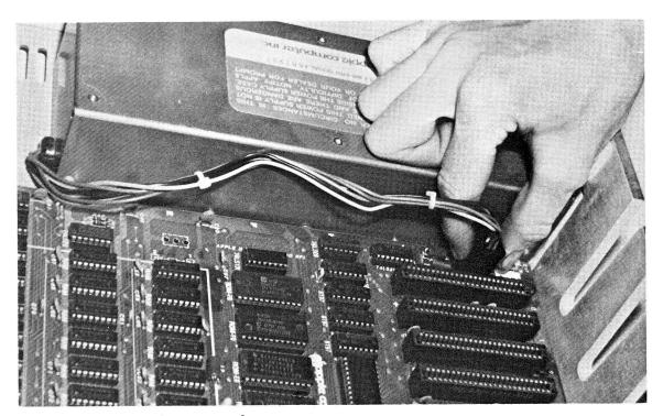
**FIG. 6–4** Location of power supply connector.
