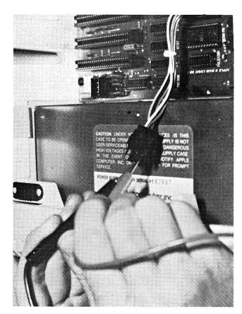
**FIG. 6-5** Checking power supply output.
