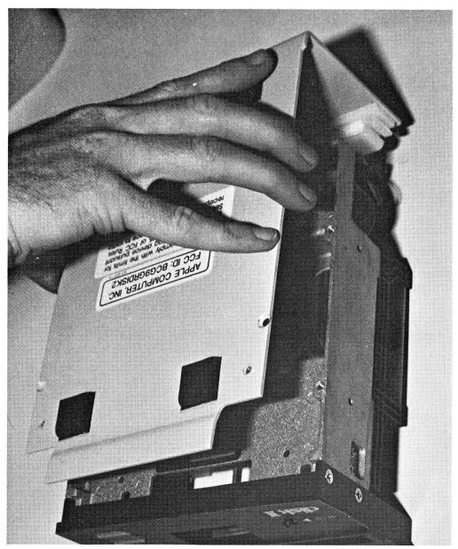
**FIG. 4–37** Lift the bottom cabinet off.
