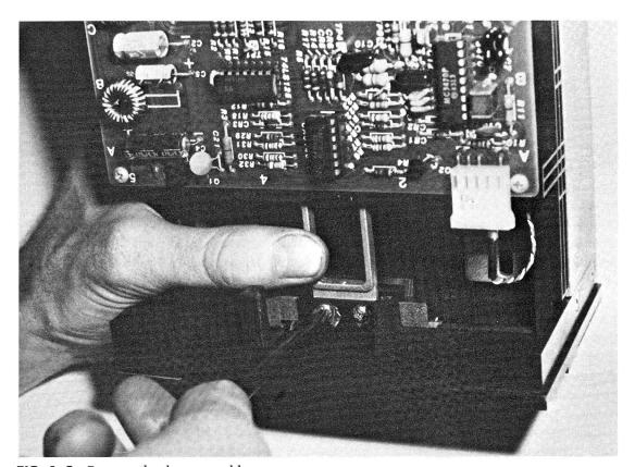
**FIG. 4–3** Remove the door assembly screws.
