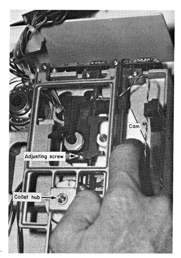
FIG. 4-9 Adjusting screw.
