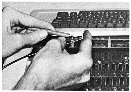
FIG. 6-8 Checking speaker continuity.
