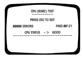
FIG. 11-5 CPU test screen.
