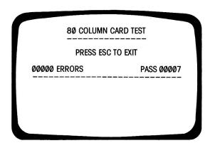
**FIG. 11–9** Eighty-column card test screen.
