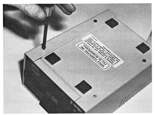
FIG. 4-29 Remove the four holding screws.
