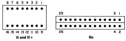
**FIG. 6–10** Pin locations on keyboard cable.
