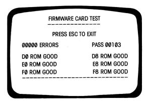
FIG. 11-10 Firmware card test screen.
