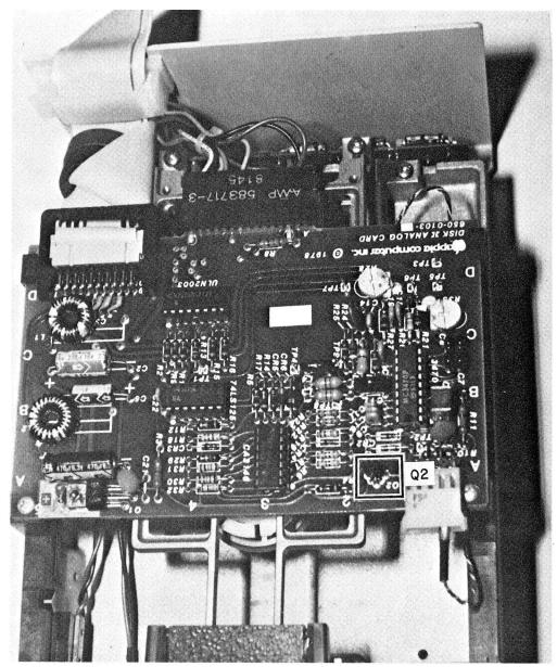
**FIG. 4–20** Location of transistor Q2.
