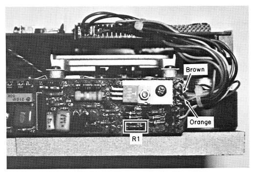
FIG. 4-16 Drive servo board.
