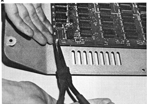
**FIG. 5–10** Removing the mother board.
