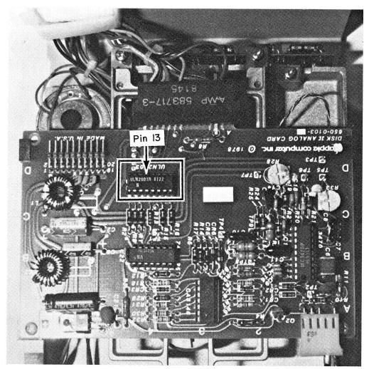
FIG. 4-18 Location of pin 13 on the ULN2003 chip.
