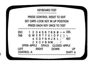
FIG. 11-14 Ille keyboard test screen.
