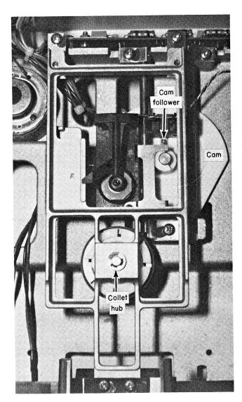
**FIG. 4–7** Carriage limiter cam, cam follower, and collet hub.
