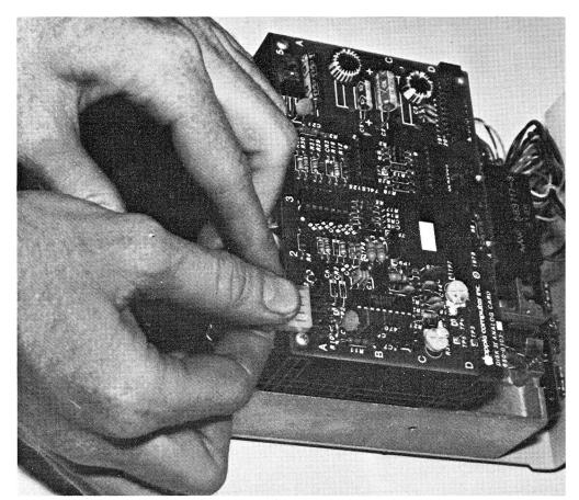
**FIG. 4–33** Remove head control cable.
