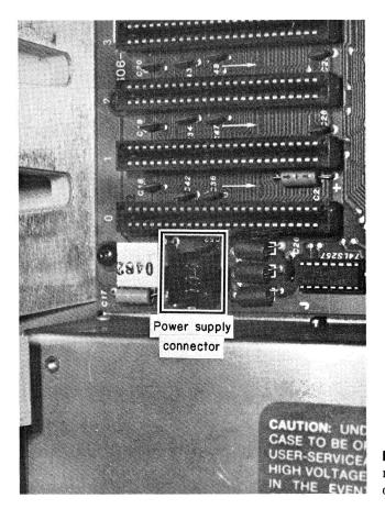
**FIG. 6–9** Location of mother board power supply connector.
