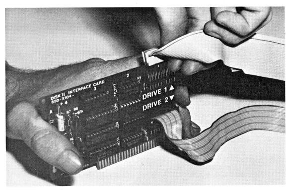
**FIG. 4–5** Swapping the drive cables.
