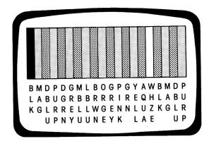
**FIG. 11–15** Color bar test screen.
