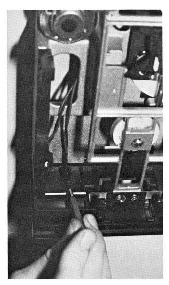
**FIG. 4–12** Replacing the drive LED.
