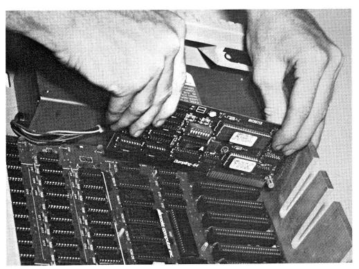
**FIG. 6–3** Disconnecting internal devices.
