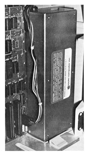
**FIG. 6–1** The power supply.
