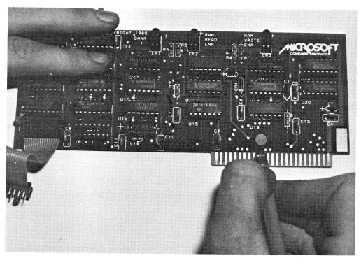
**FIG. 6–12** Cleaning the contacts of a board.
