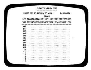
FIG. 11-18 Diskette verify test screen.
