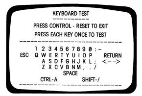
FIG. 11-13 II and II+ keyboard test screen.
