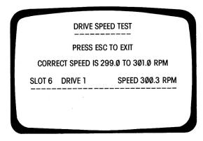
**FIG. 11–17** Drive speed test screen.
