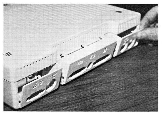
FIG. 10-3 Removing the rear panel.
