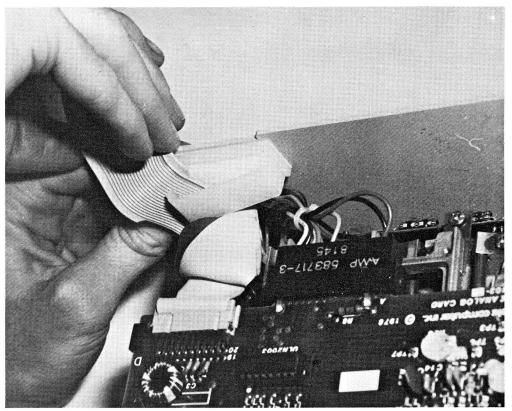
FIG. 4-31 Remove signal cable from clamp.
