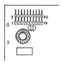
**FIG. 4–15** Pin locations on drive I/O.
