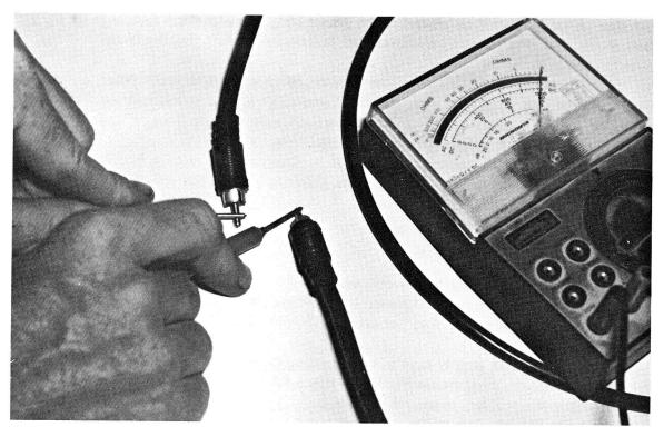
FIG. 6-11 Testing monitor cable for continuity.
