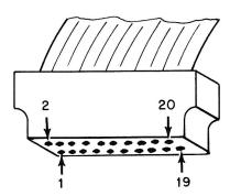
**FIG. 4–25** Pin locations on drive signal cable.
