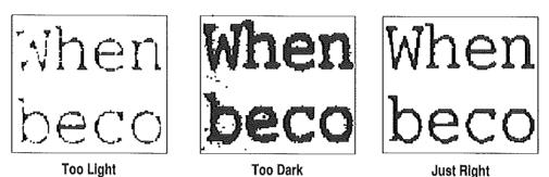
If necessary, adjust the Light/Dark thumbwheel (the wheel is very sensitive, so don't move it too far in either direction - a slight movement will do), then use the **Redo scan** command  $\bigcirc$ -R to make a new scan. You can repeat this process as many times as you like, so take your time and experiment with different settings until you get a feel for adjusting the Light/Dark control.
