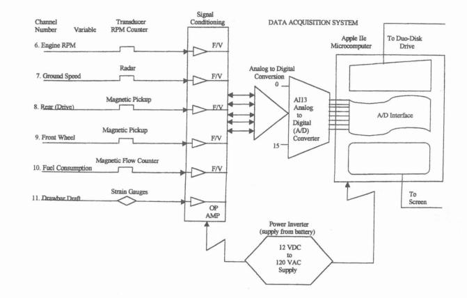
Fig 1. Block diagram of the data acquisition system hardware
