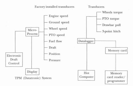
Fig 2. Block diagram of the tractor instrumentation system
