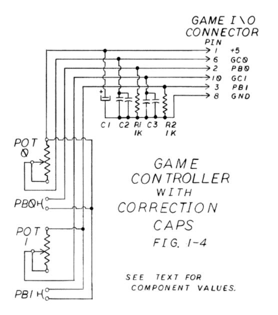
The timing circuit can be adjusted for pot values lower than the original values. This adjustment can be made by adding small capacitors within the paddle and thus requires no modification of the host computer. Figure 1-4 shows how the correction caps can be added to a standard controller circuit.
