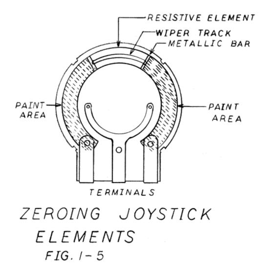
Now the pot element should look like figure 1-5. Note that there is a small active area of resistive element in the middle and two large inactive areas on either side. The problem is that the inactive areas have too much resistance to read as zero. Look closely at the limits of the wiper track, which leaves a mark, in the active area.
