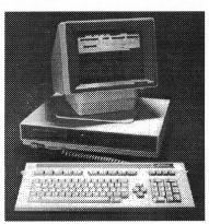
Monroe's System 2000 is a 16-bit desktop computer built around Intel's new 80186 microprocessor operating at 8 MHz. For 8-bit compatibility, the 2000 can be optionally equipped with a Z80A alternate processor. The computer is supplied with 128K or 256K of RAM, optionally expandable to 896K, exclusive of the 128K used for monochrome or 192K used for RGB color video display. The computer comes with one or two 51/4" floppy disk drives, each with a capacity of 640K (CP/M-86)/720K (MS-DOS).
